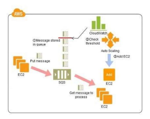
Refer to the architecture diagram above of a batch processing solution using Simple Queue Service (SOS) to set up a message queue between EC2 instances which are used as batch processors Cloud Watch monitors the number of Job requests (queued
