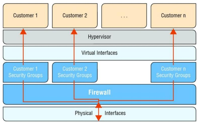
FIGURE 12.3 Amazon EC2 multiple layers of security
