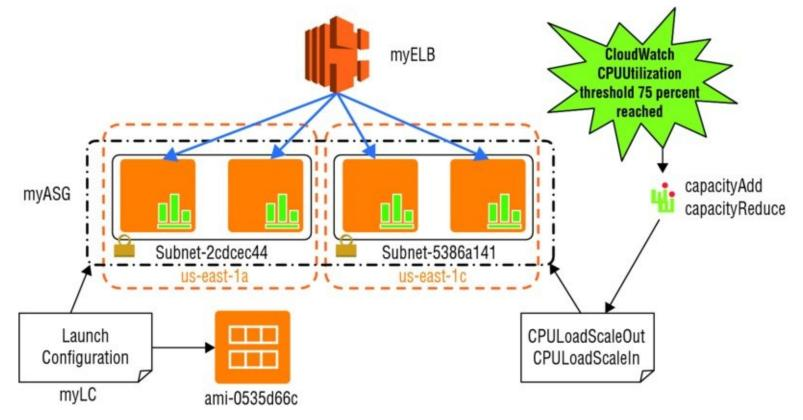
FIGURE 5.3 Amazon CloudWatch alarm triggering scaling out
