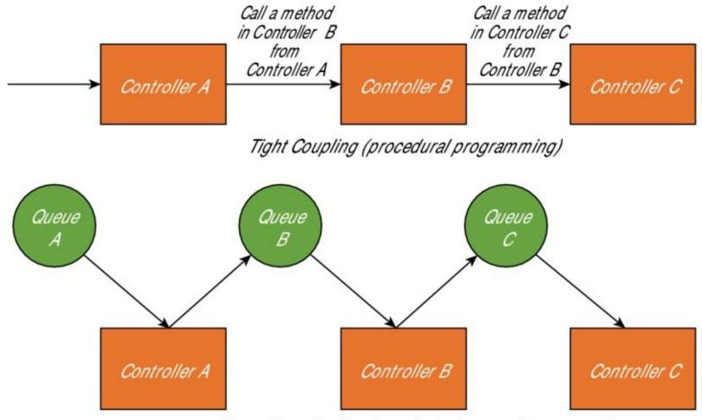
Loose Coupling (in dependent phases using queues )
