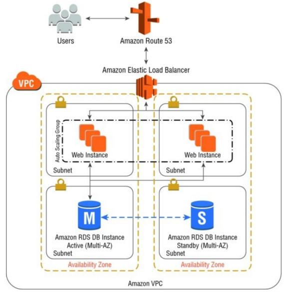
FIGURE 14.3 Updated web application architecture with auto scaling
