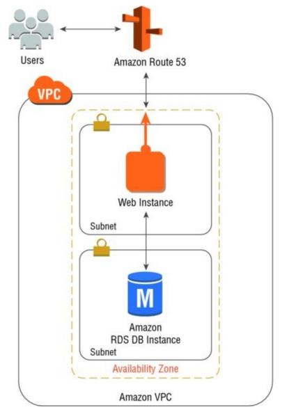
**FIGURE 14.1** Simple web application architecture
