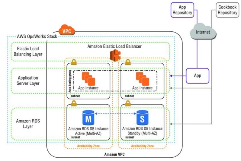
**FIGURE 11.7** Simple application server stack with AWS OpsWorks
